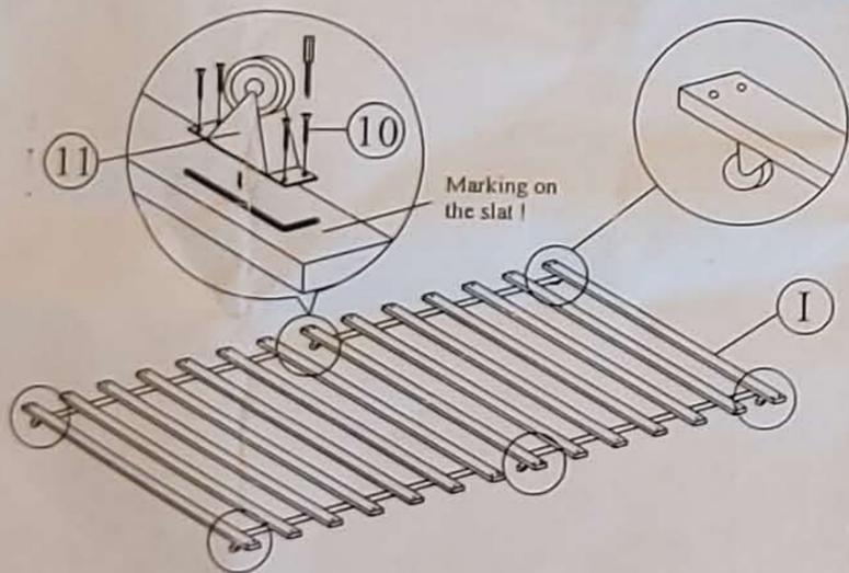
Step 6: Place the wooden blocks (J) at the corner of the trundle and fix the slat (I) to the side rail at (F) & (G).
