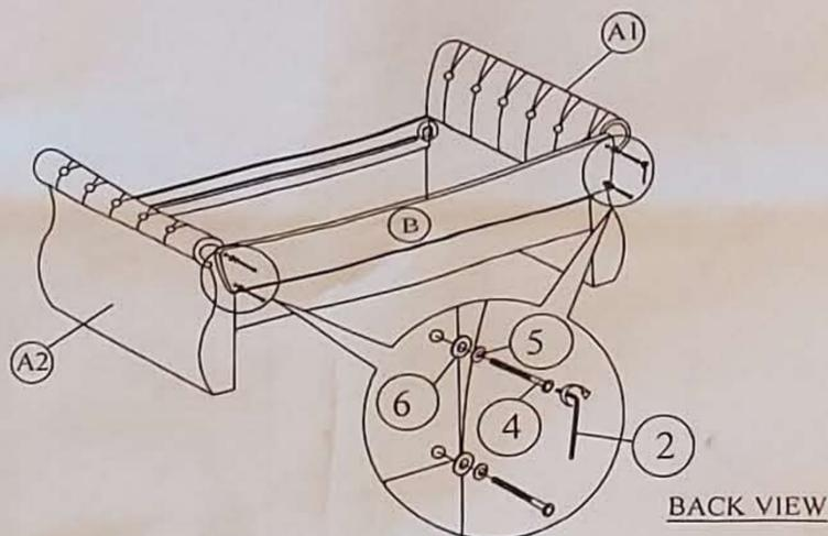
Step 3: Tighten the 4 Corner with Allen Key (1). Install the slats to side rail. Tighten the slats with CSK screw (3). The distance of the slats should be sufficient to obtain desirable bed stability.
